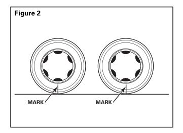
6. Turn the forward driveshaft in one direction by hand until the forward tire completes two rotations. Ensure that the forward tire rotates two times only. If the forward tire rotates more than or less than two rotations, the angle measurements you make in Step 7 will be inaccurate.
