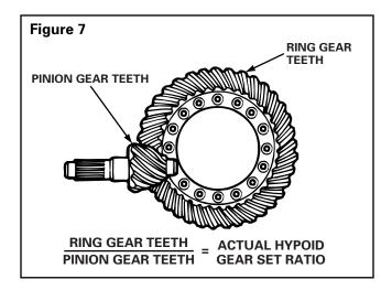
Calculate the percentage difference between the hypoid gear set ratios using the equation below. All ratios must match within one percent.
