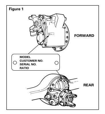
2. Compare the axle ratios shown on both tags. To operate correctly, the axle ratios for both axles must be within one percent of each other. To calculate the percentage difference between the axle ratios, refer to the equation below.
